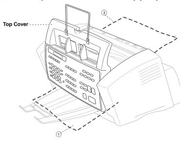
2 Lift the top cover and make sure where the paper is jammed.
